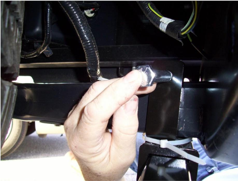
**Step 2.** Install the hex bolt in the cross holes of the u-bracket, as shown at left. Please note that the bolt can be installed in either direction. Back to front is shown.
