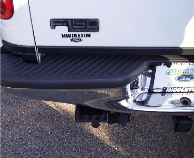
DEBO Step Installed, Stowed Position
