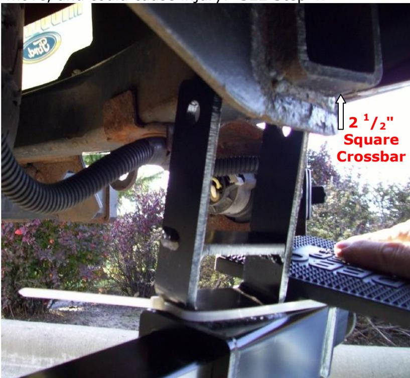
**Step 1.** The DEBO Step mounts on the driver's side of your truck, on the hitch frame cross bar.
