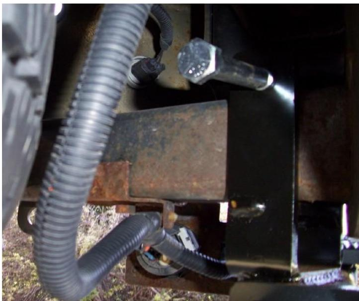
**Step 2.** Install the hex bolt in the cross holes of the u-bracket, as shown at left.
